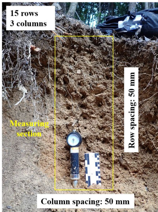
Fig. 11 Hardness test of the in situ soils at the DF3 source area: a testing ranges and b tested results of unconfined compressive strength along the depth
