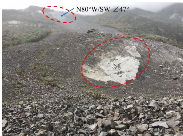
Fig. 7 Bedding planes observed at the scarp and failure surface of the Xinmo village rock avalanche in 2017. Photo from Hengxing Lan, 5 September 2018
