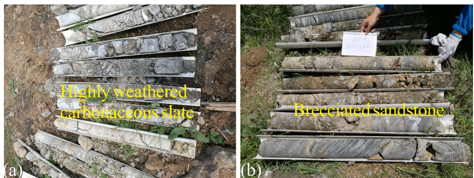
Fig. 18 Inferred failure surface for K2-1 and K3-1: a highly weathered carbonaceous slate at depth of 15 m in ZK 17 and b brecciated sandstone at depth of 19–21 m in ZK 18
