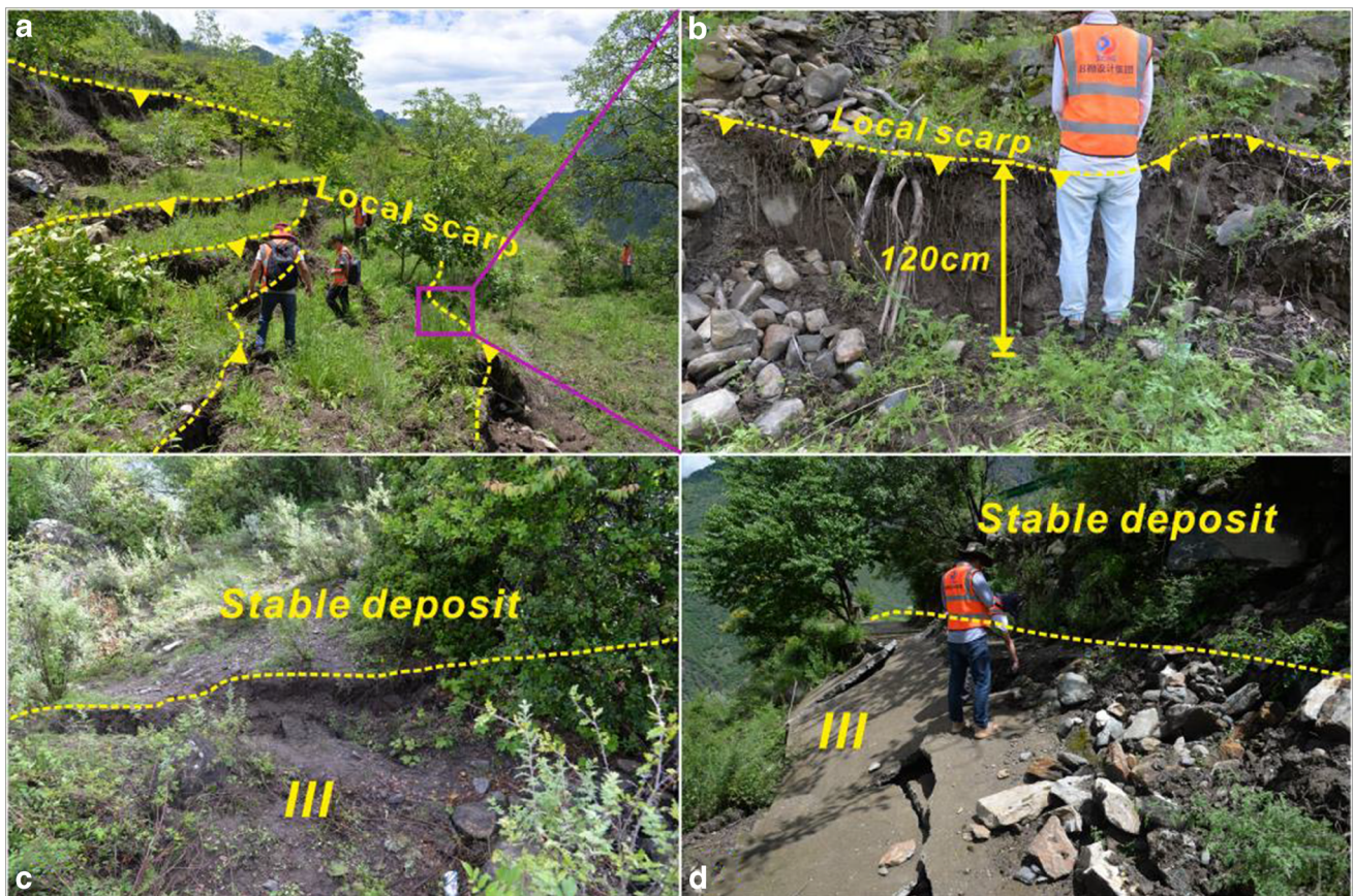
Fig. 14 The boundary characteristics of upstream deformation zone III. a, b Local multistage scarps in zone III. c, d Characteristics of the upstream boundary. The locations of a, c, and d are listed in Fig. 9
