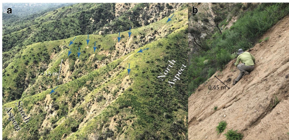
Fig. 8 a Photo showing shallow landslides in the study area. Blue arrows indicate landslide scarps. b View near the scarp of one landslide with the depth of the landslide release zone indicated (photo credit. F. Rengers)
