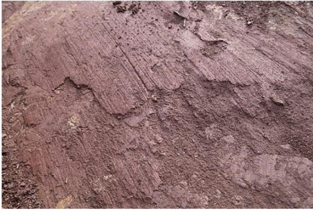
Fig. 13 The remaining fuchsia slip zone on the sliding bed-yellow sandstone surface, with a large area of polished surface and striated scratches on the slip zone (photo taken by Bolin Huang after failed)
