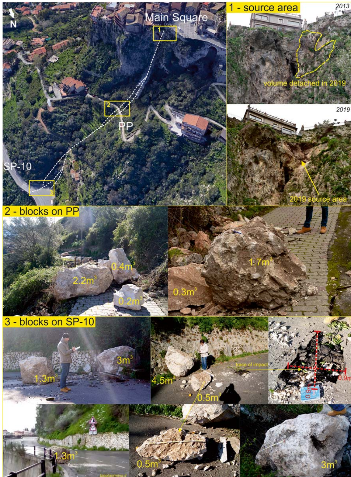
Fig. 3 Reconstruction of the rockfall trajectory with a focus on the three key spots: 1, source area with a comparison between photos taken in 2013 and 2019; 2, surveyed blocks along PP; 3, surveyed blocks along SP-10
