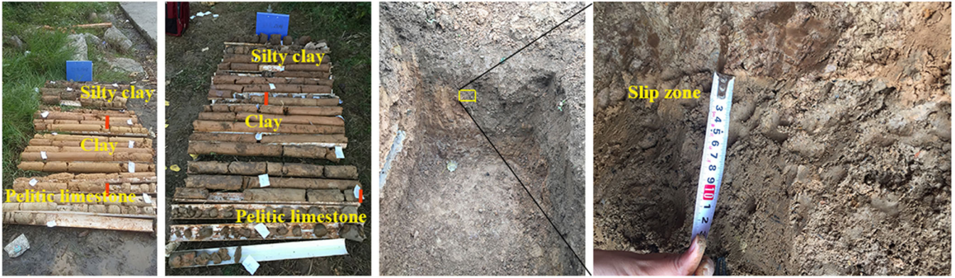
Fig. 5 Lithological stratigraphic logs of boreholes (B02 and B05) and the slip zone of the Linjiabang landslide exposed by exploratory trench
