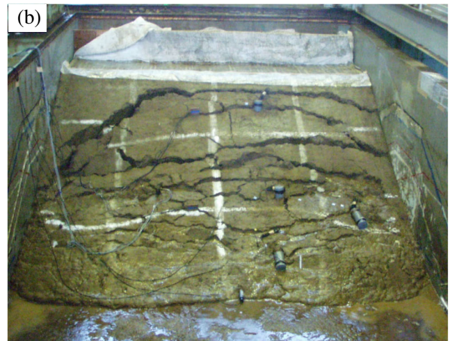
Fig. 13 Images of big scale model test: (a) The image of the slope before failure, (b) The image of the slope after failure
