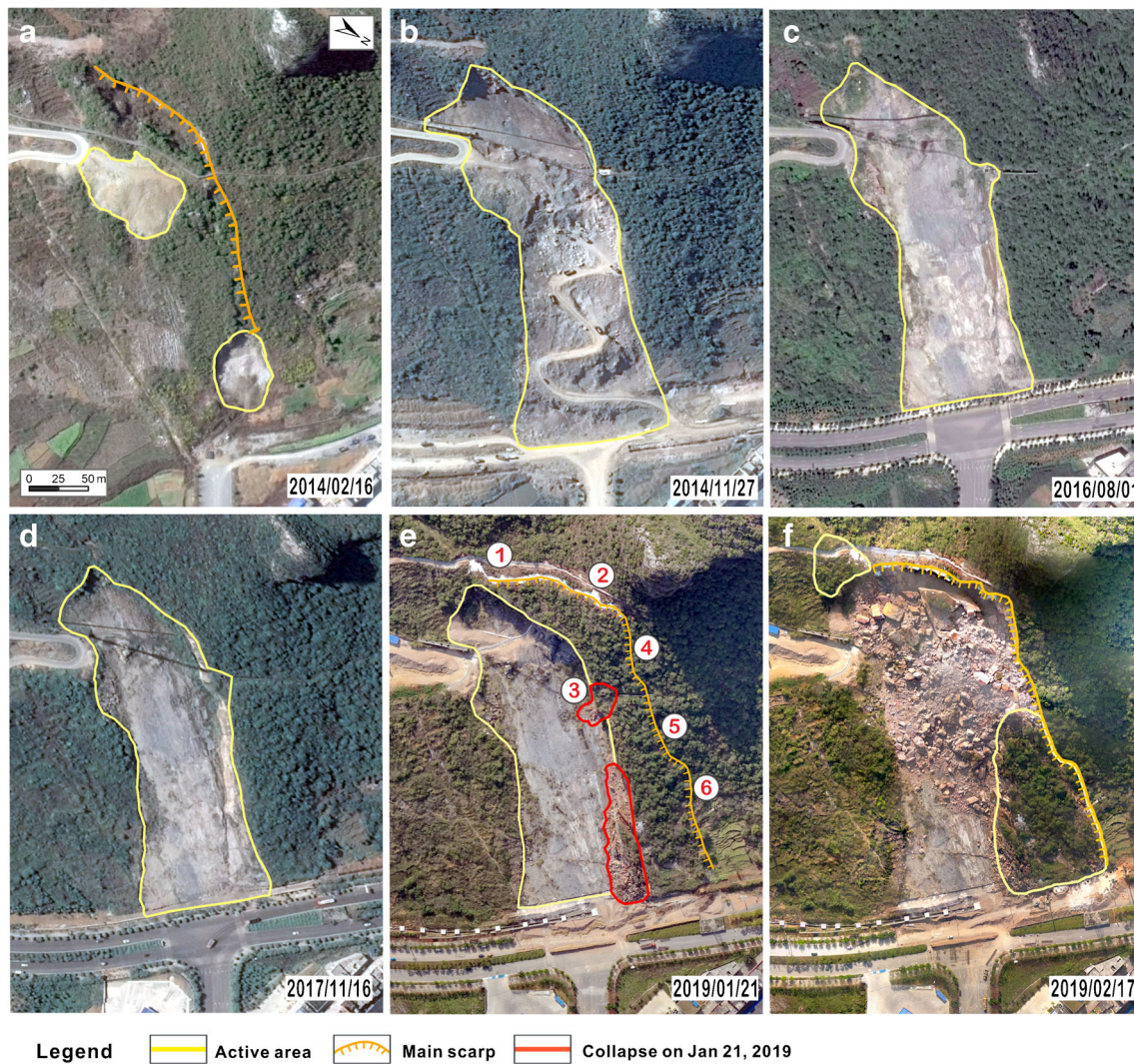
Fig. 4 Visual interpretation of historical deformation of the rockslide from Google Earth images (the date is shown using YYYY/MM/DD format), a 2014/02/16, b 2014/11/27, c 2016/08/01, d 2017/11/16, e 2019/01/21, and f 2019/02/17. The numbers (1), (2), (3), (4), (5), and (6) in (e) are locations of photographs (see Fig. 5) taken along the orange scarp line
