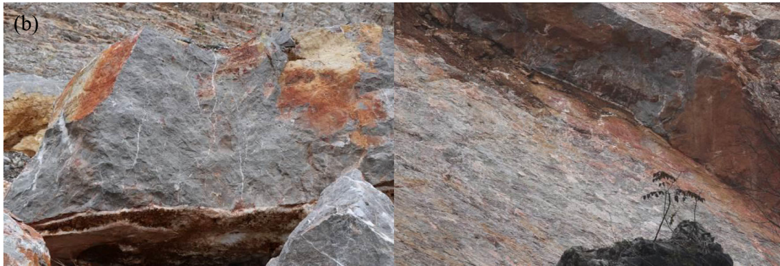
Fig. 3 The geological conditions of the bedding rockslide. a The situations of stratum; b the calcites filled in the joints surface
