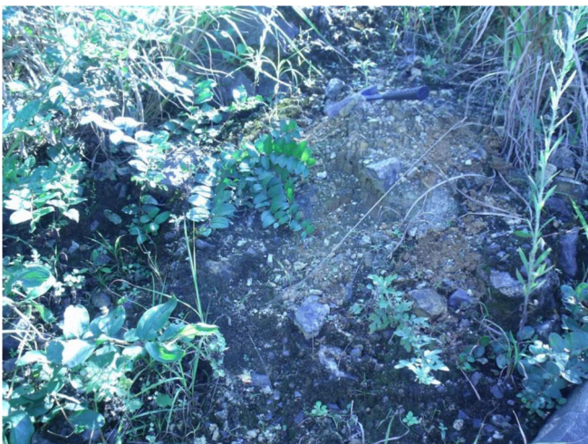
Fig. 7 Deposit at point D in Fig. 2, over 5 years after the event. The hammer (near the top) is about 30 cm in length. Yellow loose soil makes up over 50% of the debris in volume, which facilitates the growth of vegetation
