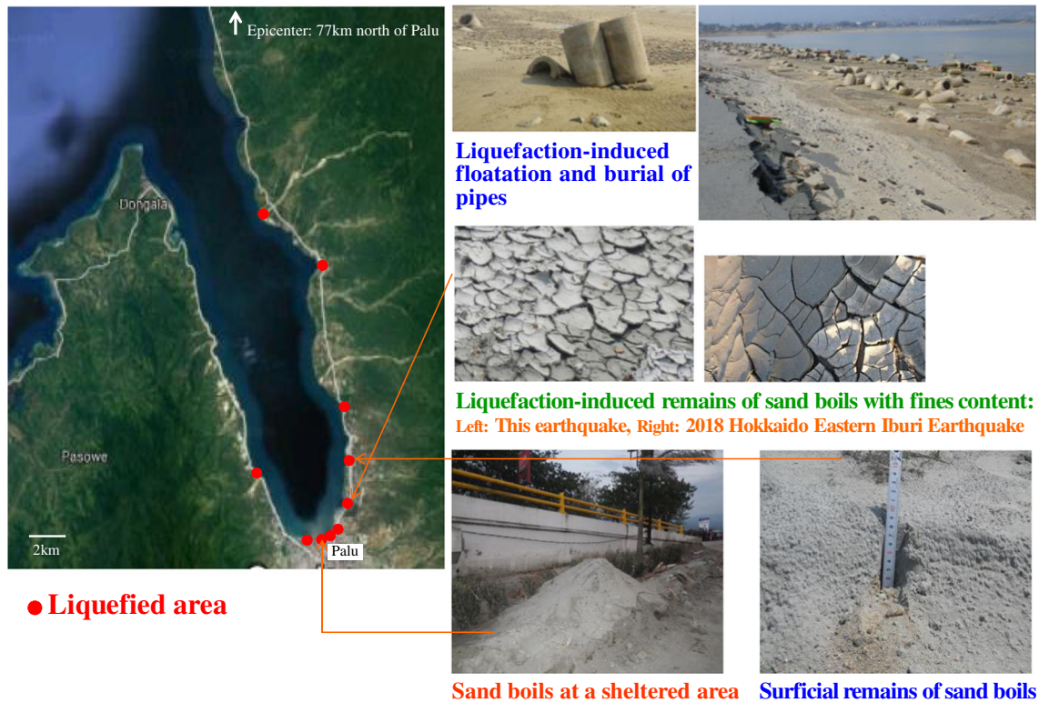
Fig. 2 Evidence of extensive coastal liquefaction along Palu coast
