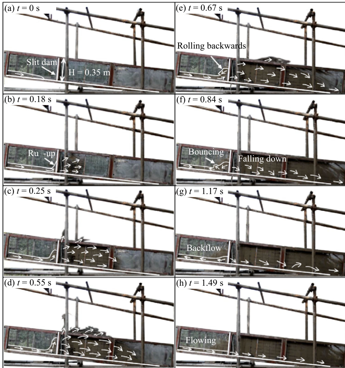
Fig. 8 Interaction process between debris flow with high water content ( W = 30\% ) and slit dam with wide relative post spacing ( b/d_{\max} = 3.1 ): test S-W30-3.1
