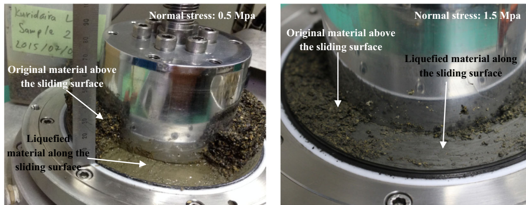
Fig. 17 Sliding surface liquefaction behavior of shale samples under different normal stresses in ring shear tests
