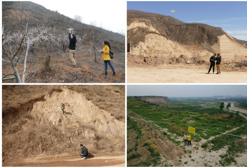
Fig. 7 Loess landslide field investigation using low-cost UAVs on the Loess Plateau
