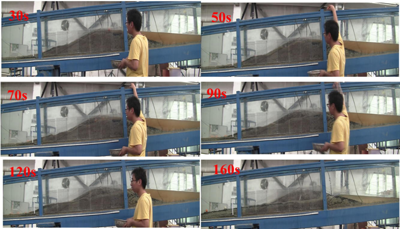
Fig. 6 Images of the dam at different times for T-5, which shows the gully deepening by overtopping erosion and the characteristic breach phases
