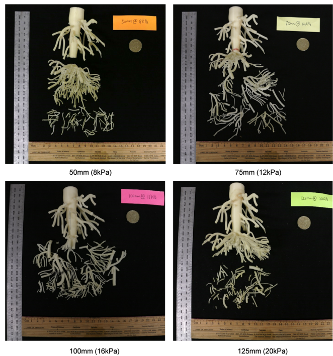
Fig. 16 Breakage of root clusters under varied confining stress following careful post-test exhumation
