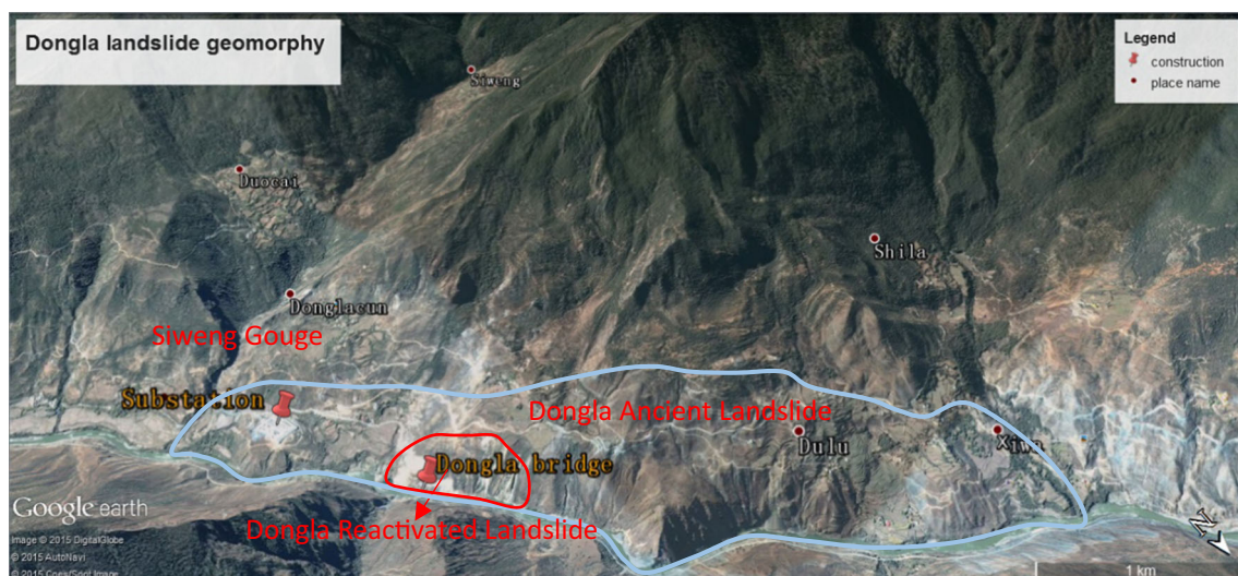
Fig. 2 Delineation of the Dongla Ancient Landslide and Dongla Reactivated Landslide
