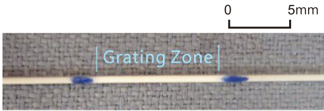
Fig. 8 Encapsulated FBG sensing fiber
