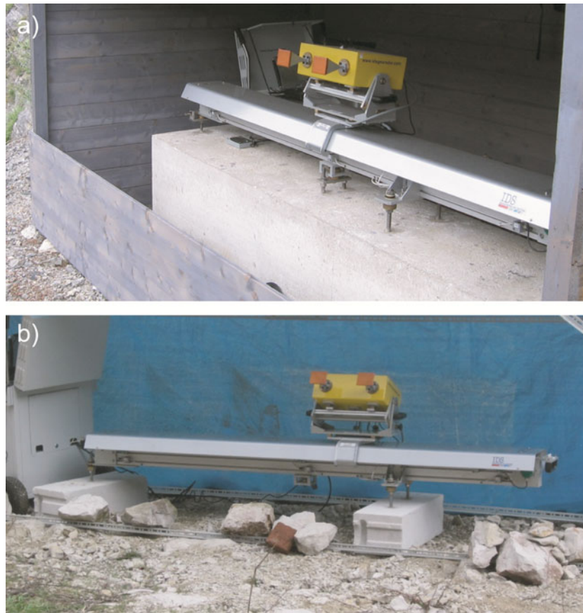
Fig. 2 Example of GBInSAR installation systems: concrete base (a); rapid installation and repositioning system (b)
