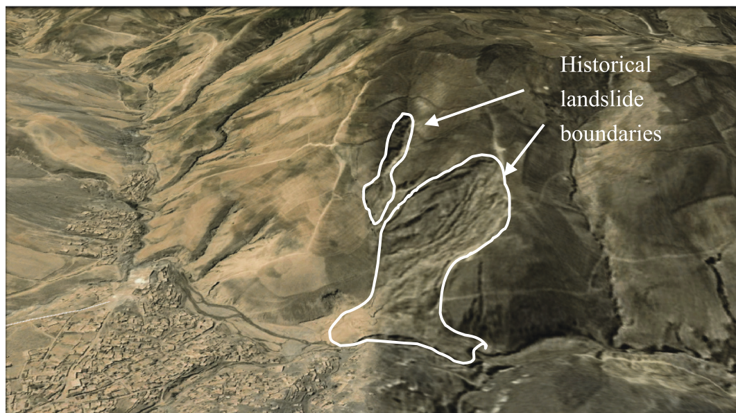
Fig. 9 Historical landslide (image: 10 July 2014, Google Earth)
