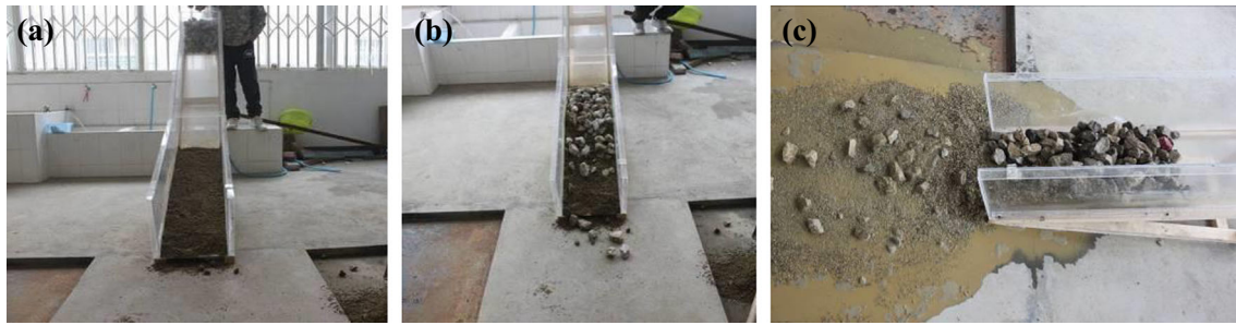
Fig. 16 Experimental results for the impact and scouring of sliding masses: a experimental preparation, b final deposited situation of test No. 6, and c final deposited situation of test No. 4
