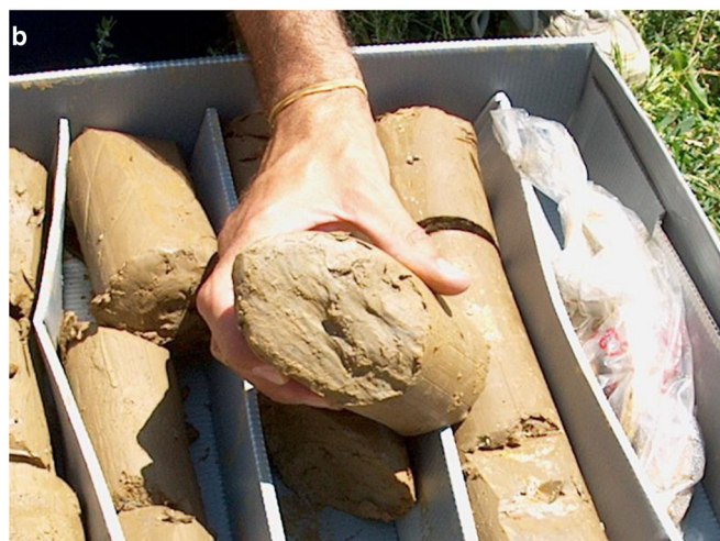
Fig. 8 Viladesens slide. a Cross section; b striated and polished surface in brown clay observed in recovered cores
