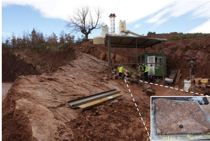
Fig. 20 Castrovido Weald form. Exposed sandstone–claystone sedimentation surface. Zoom-in of contact after in situ shearing test
