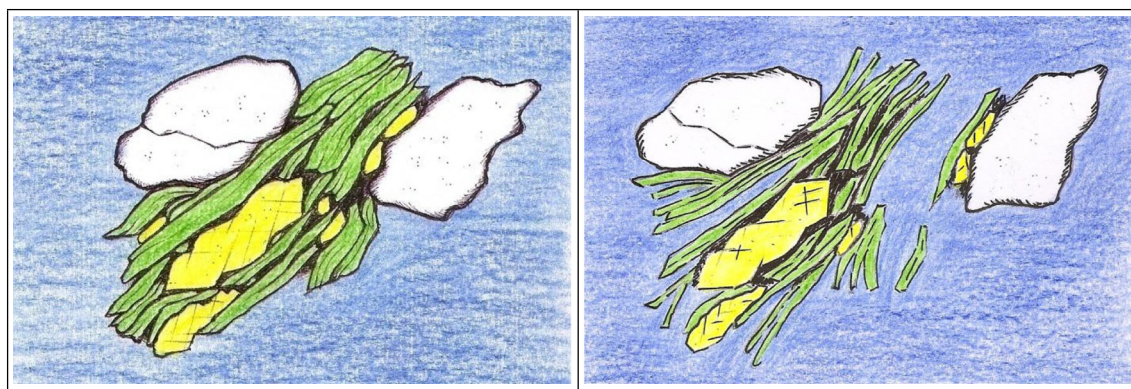
Fig. 20 Interpretative sketch of the rock disaggregation. Left : sand-size calcite crystals ( yellow ) bonding both clasts ( white ) and phyllosilicates ( green ). Right : disaggregation of the rock is facilitated by the presence of weak phyllosilicate layers bonds
