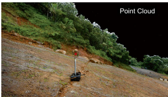
Fig. 9 Colored TLS point clouds showing a pair of collocated GPS antenna and reflector (red round panel) installed for TLS survey
