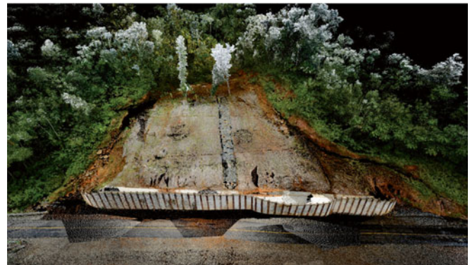
Fig. 8 Colored point clouds collected by TLS (RIGEL VZ-400) on 25 May 2010 during the first TLS survey
