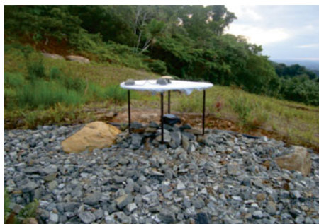
Fig. 6 Images showing the ground target in the middle of Fig. 5 and the laser points hit on the surface of the ground target. Note that the GPS antenna and rocks were not on the table during the airborne LIDAR surveying period. The unit of the scale in the right figure is meter
