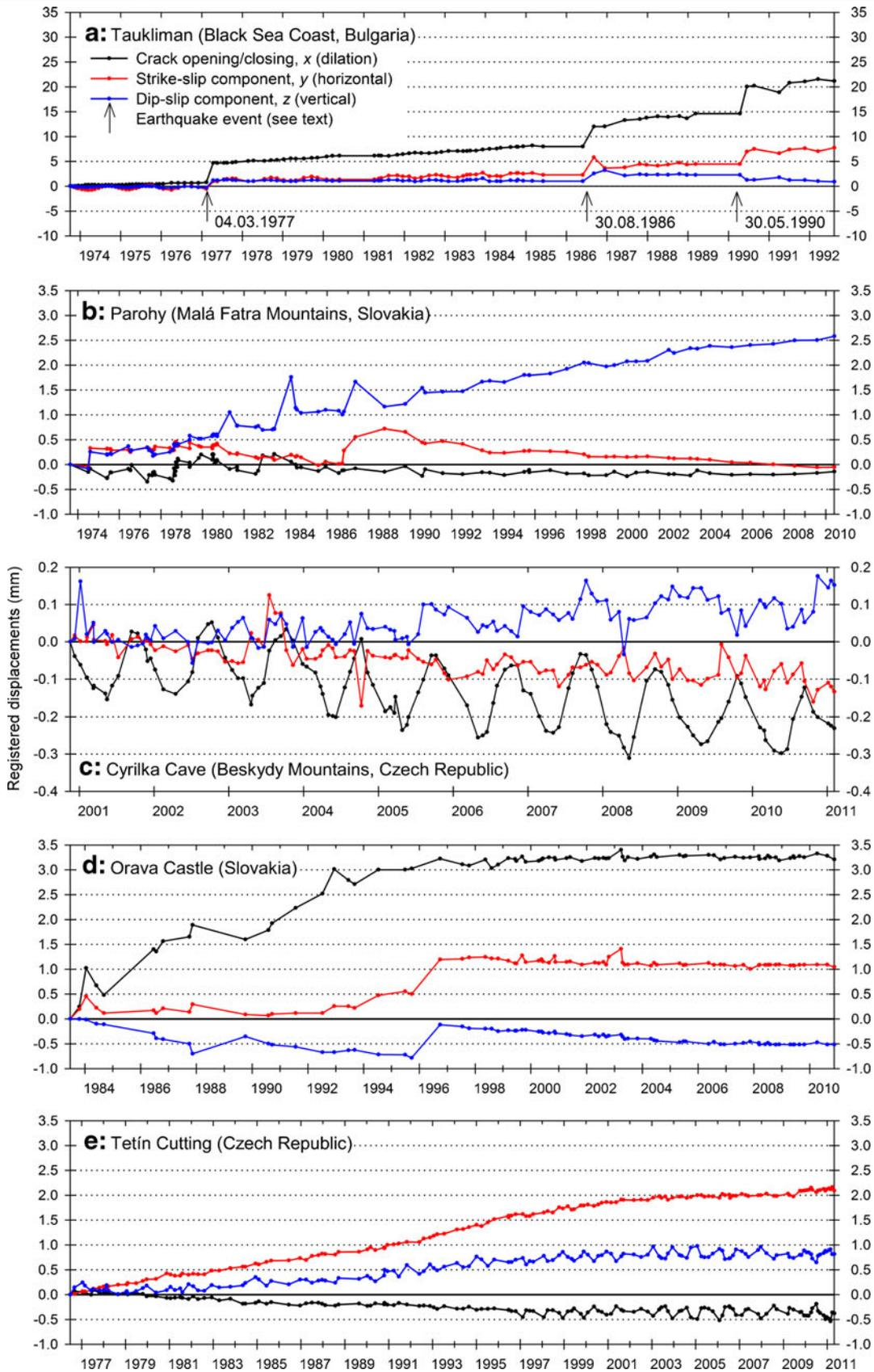
**Fig. 3** The optical-mechanical crack gauge measurement results at the selected sites. Note the changes in scale on both the x- and y-axes
