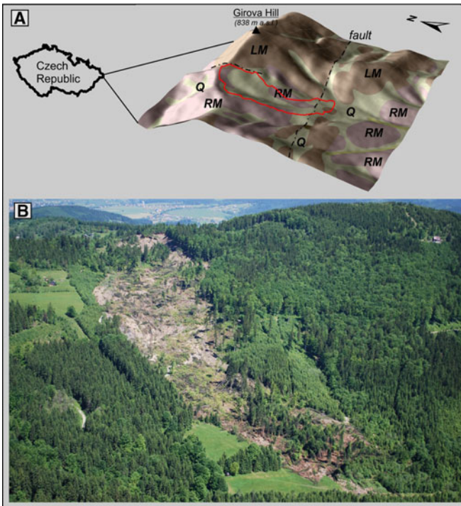
Fig. 1 General setting of the Gírová landslide area: a 3D Visualization of the geological map from SW. Q quaternary slope deposit, RM Raztoka Member, LM Lukov Member (Source of data: ZABAGED and Czech Geological Survey); b oblique aerial photo of the Gírová landslide from S (Photo by I. Baroň; June 5, 2010)
