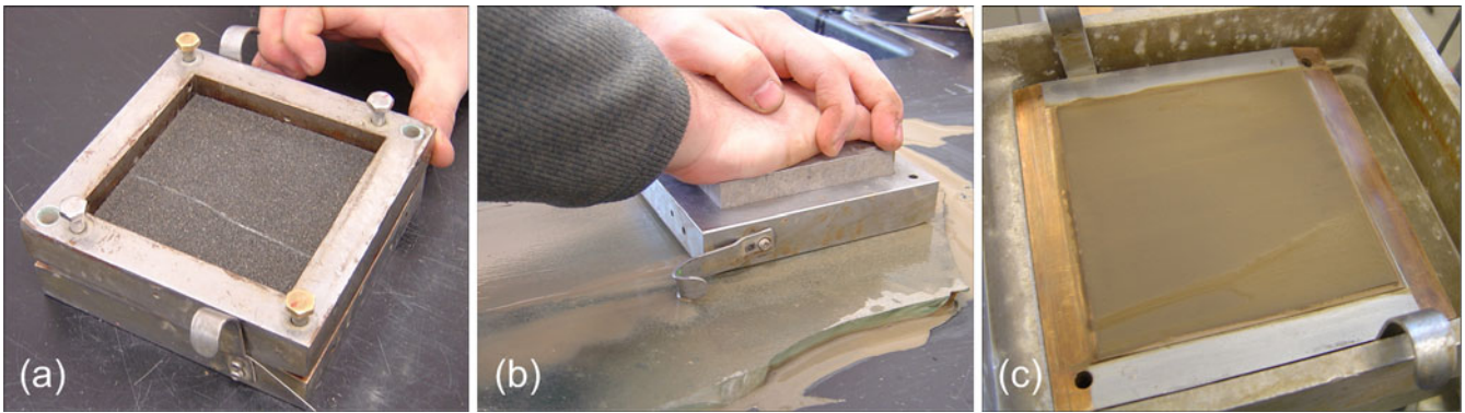
Fig. 5 Preparing a direct shear test specimen; a wire-cutting a direct shear specimen, b rubbing the cut plane on frosted glass to align clay particles, c the polished failure plane
