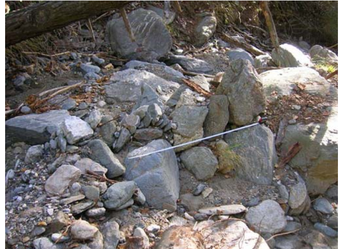
Fig. 8 Example of a train boulder in a debris flow along the T. Secco (G3 type); the white tape is 1 m long
