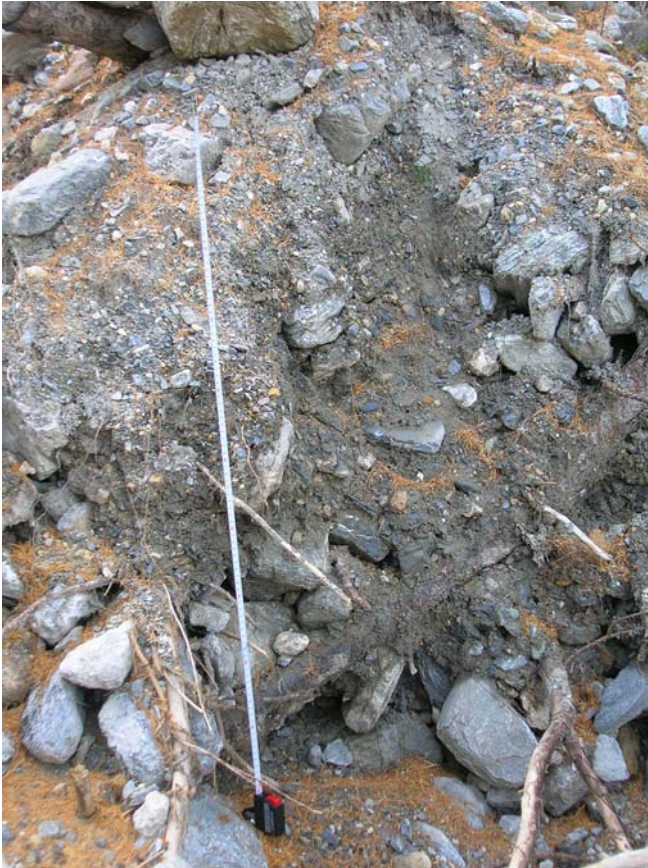
Fig. 6 Example of debris-flow deposit in G1 type basin (R. C. Gorgia); the white tape is 1 m long
