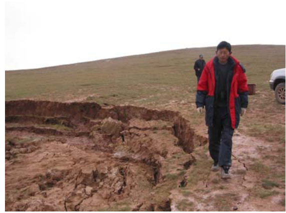
Fig. 6 The head-scarp of the thaw slump at K3035 of the Qinghai-Tibet Highway
