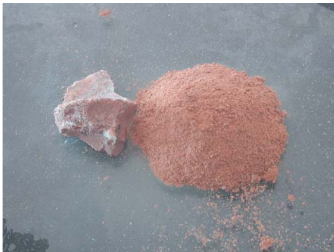
Fig. 7 Stability of conglomerate ( left ) and degradation of siltstone ( right ) after only a few minutes of immersion in water
