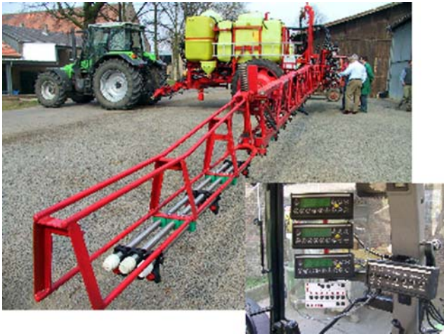
Fig. 5 GPS-controlled patch sprayer with three separated hydraulic circuits
