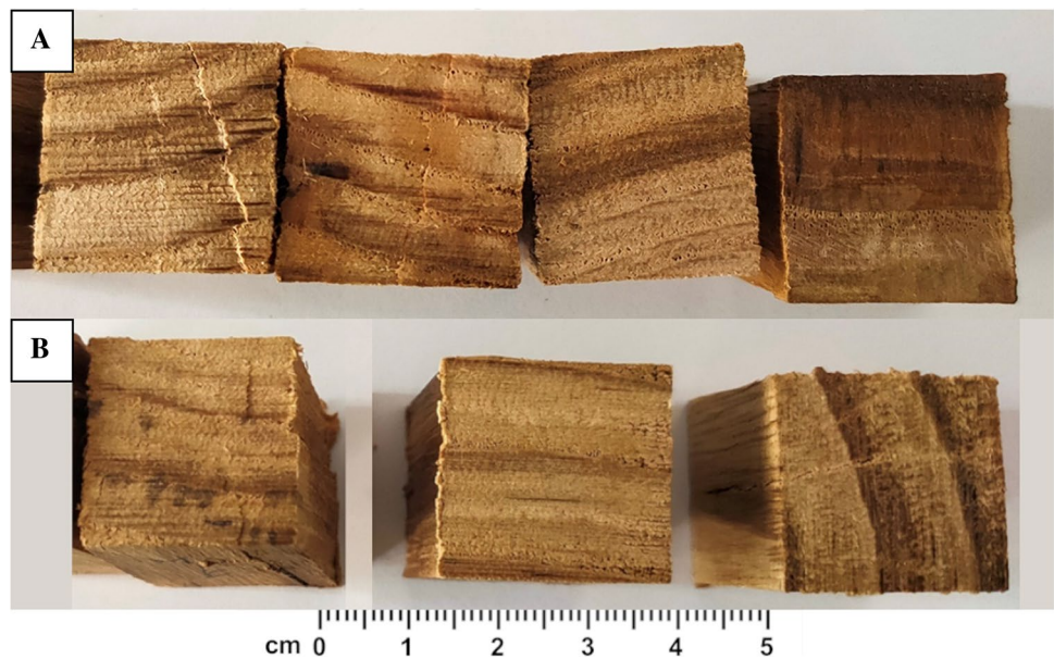
Fig. 4 a Test samples from the fourth quartile (Q4) of both G1 and G3, with strong colour alteration. b Test samples from the first quartile (Q1) with high compressive strength with colour aberration as well
