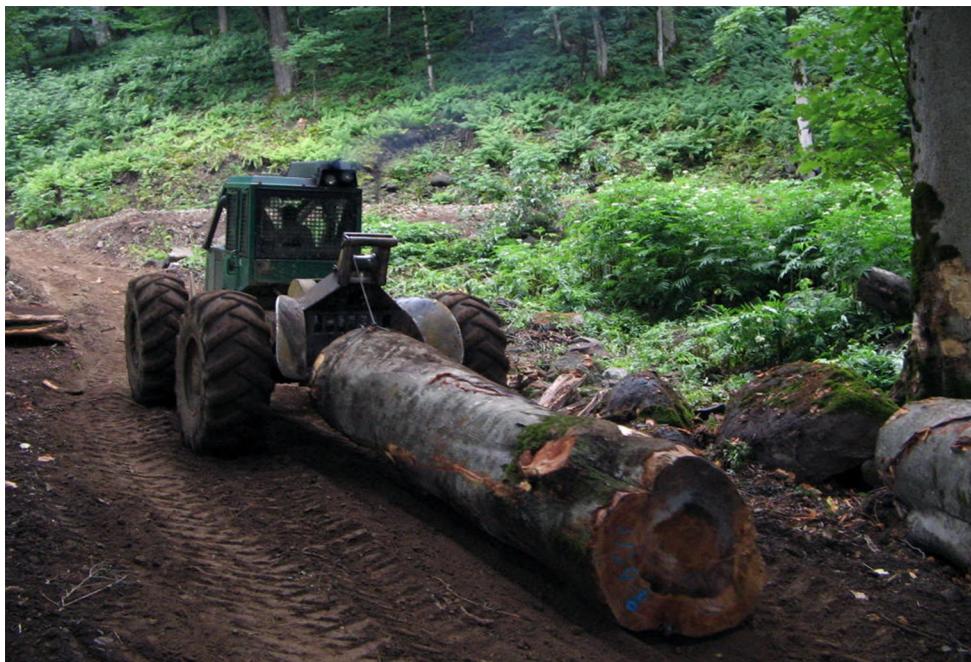
Fig. 1 Rubber-tired cable skidder (Timberjack 450C) used for logging operations in a mountain forest of Iran
