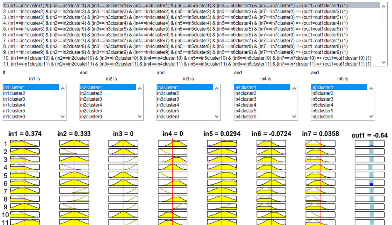
Fig. 6 Table of rules and working steps for the fuzzy inference system of our adaptive neuro-fuzzy interface system model
