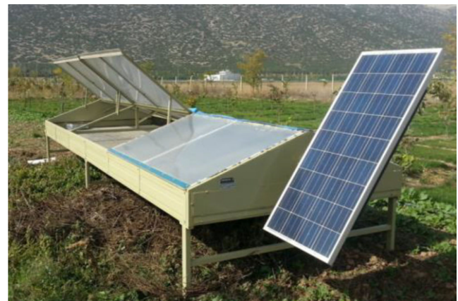
Fig. 1 The experimental solar tunnel dryer
