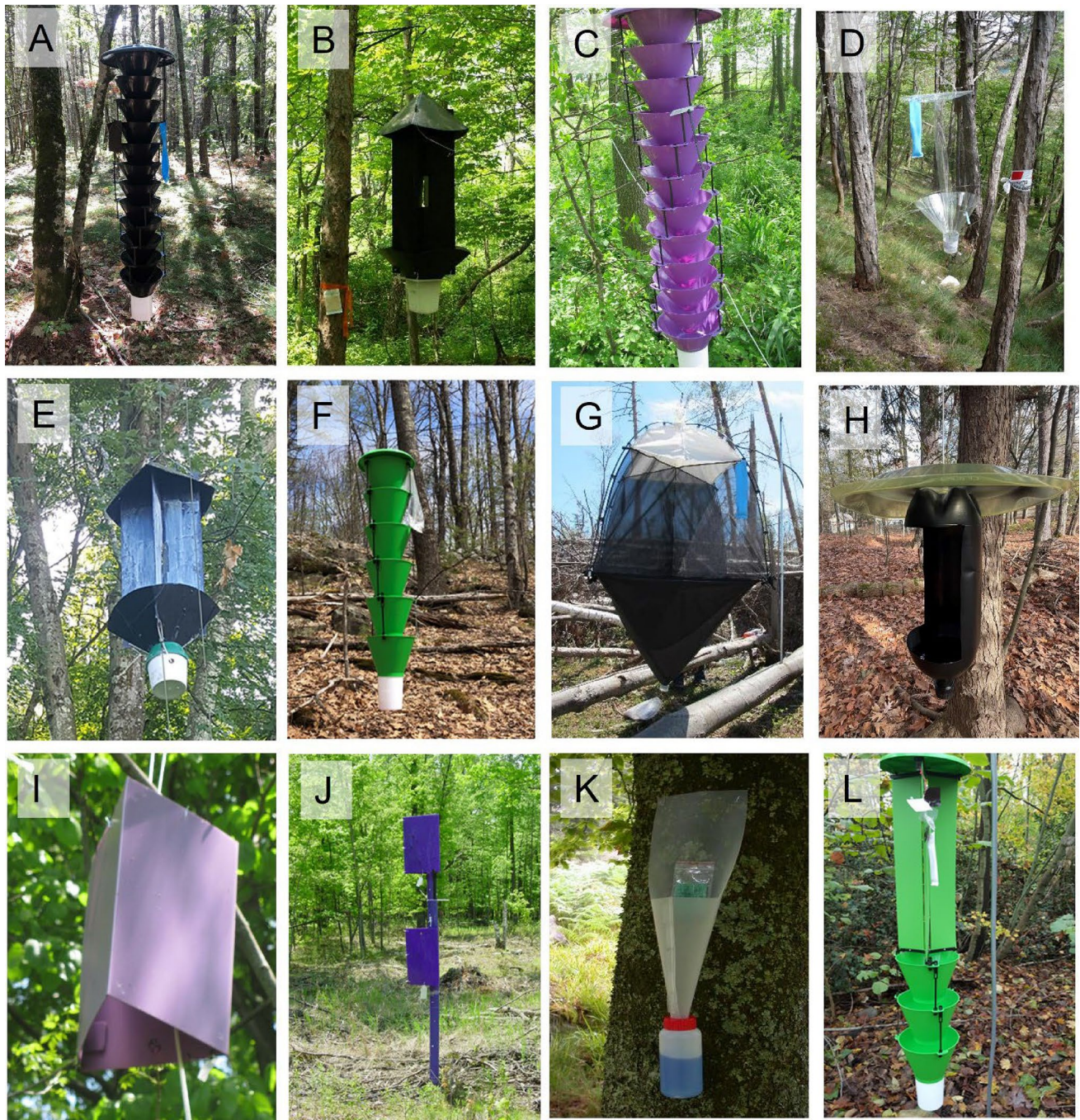
Fig. 2 Trap types used to survey bark beetles and woodboring beetles for various purposes. Traps include multiple-funnel (A), intercept panel (B), purple multiple-funnel (C), transparent intercept panel (D), fluon coated intercept panel (E), green multiple-funnel with enlarged funnels and collecting cup (F), SLAM aerial malaise (G), bottle (H),
