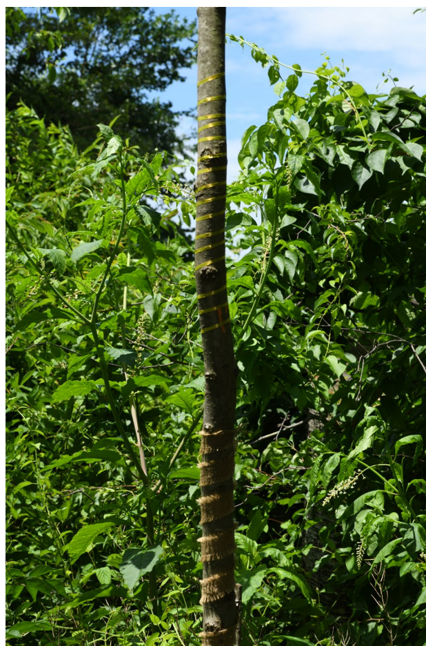
Fig. 1 Burlap trap (0.03 m × 1 m) and polypropylene ribbon trap (0.005 m × 2 m) were installed as spiraling wraps on the main trunk of a white ash tree
