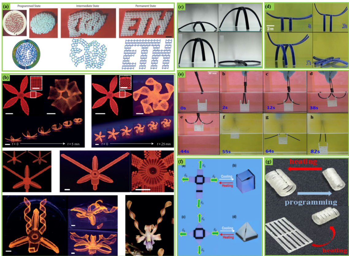
Fig. 14. 2D printed structure from 2D to 3D deformation: a 2D deformable honeycomb structure [120]; b 2D planar structure twists, bends, and deforms, then assembles into flowers [121]; c smart trestle [112]; d smart insect-like structure [112]; e smart hook [112]; f foldable cartons and pyramids [118]; g automatic curling hinges [122]
