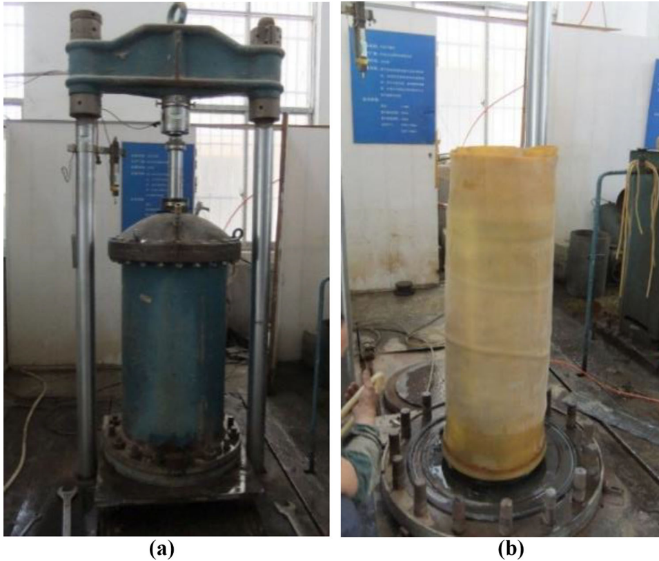
Fig. 2. Large-scale triaxial compression test: a triaxial apparatus; b specimen
