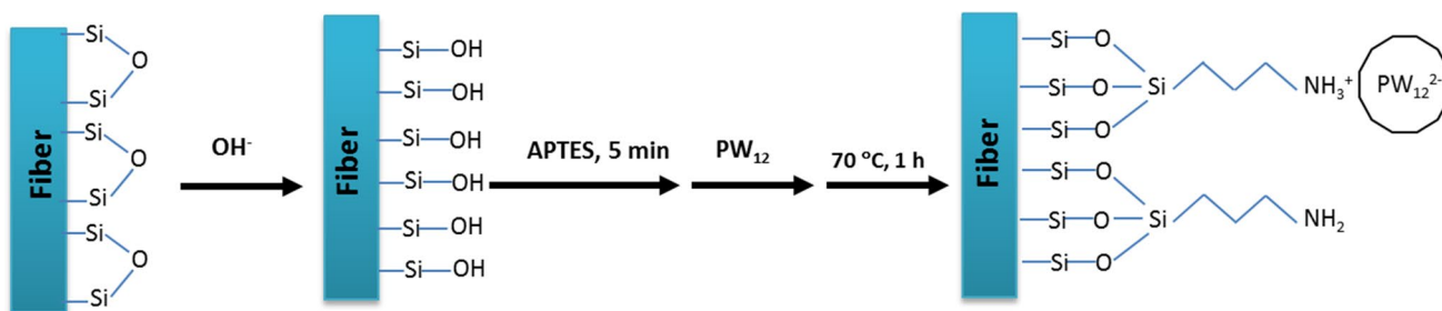
Fig. 2 Schematic illustration of the preparation process for the PW12-APTES@fiber
