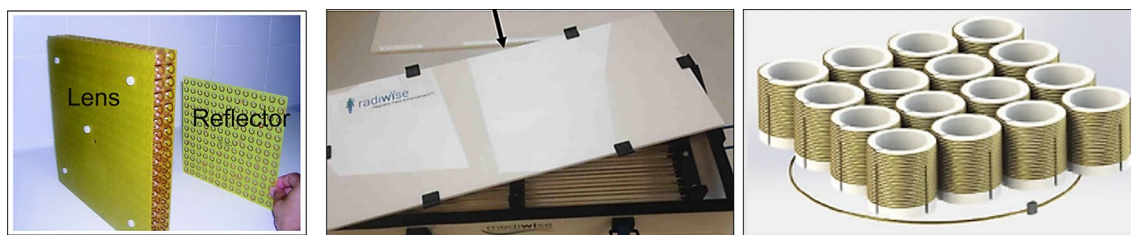
Fig. 12 Photographs of various metamaterial-based prototypes for MRI. (Left) A metamaterial lens based on split rings [61], (centre) a structure based on conductive rods within a high permittivity liquid
