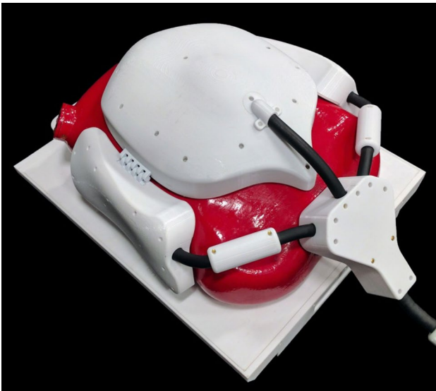
Fig. 7 Array coil posed on the anthropomorphic to-scale gravid uterus phantom used by Spatz [36]
