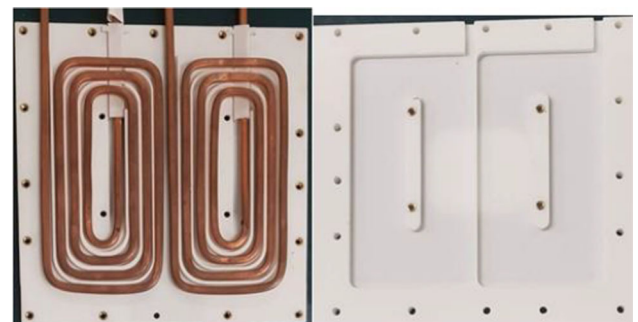
Figure 2. Manufactured X-coil using OFHC Copper hollow tube and fixing polyamide structure.
