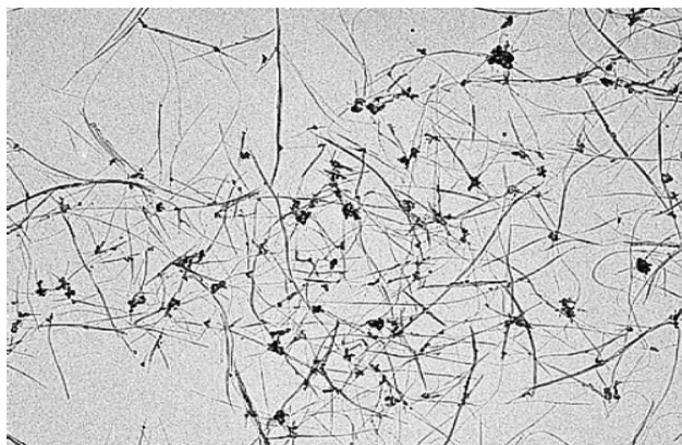
Fig. 7 TEM photograph of imogolite fiber. Allophane aggregates are also present. Bar indicates 200 \mu\text{m} (Shimura et al. 2012)
