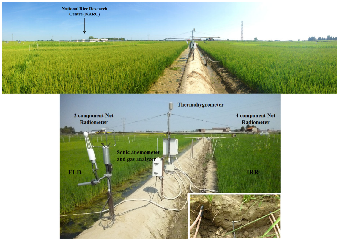
Fig. 3 Pan of the rice fields and zoom on the eddy covariance station mounted on the levee between FLD and IRR treatments. In the bottom right box , the installation of four thermistors and a soil heat flux plate
