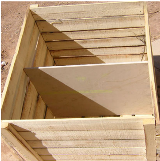
Fig. 1 Wooden box and the thin plate inside it for PRD experiments
