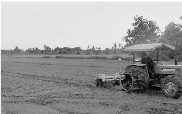
Fig. 2 Veris 3100 sensor cart pulled behind a tractor across a paddy field
