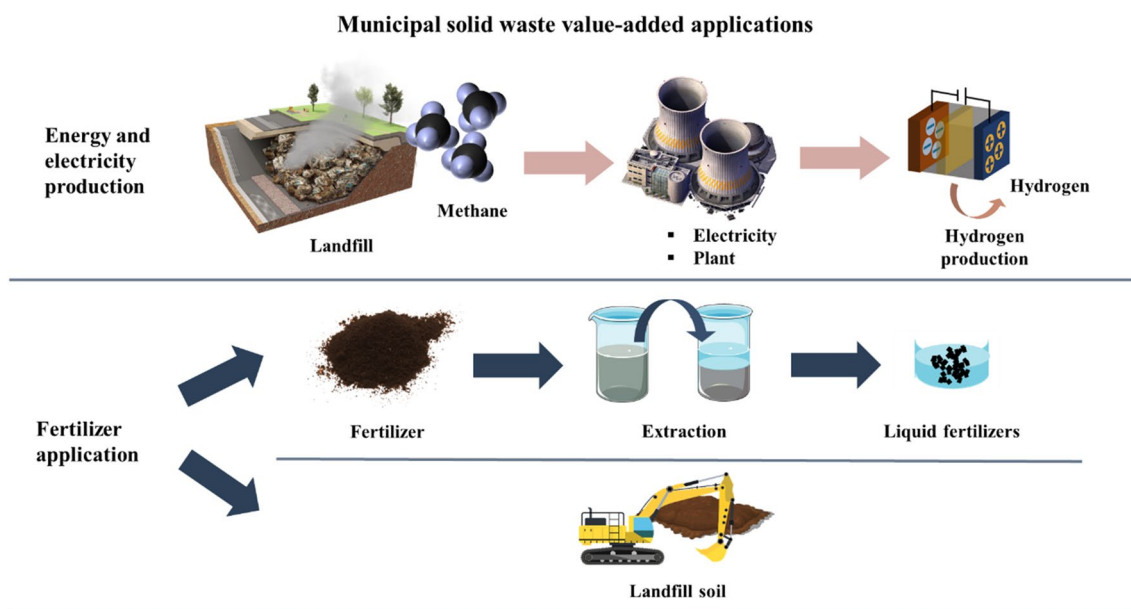
Fig. 2 Municipal solid waste value-added applications. There are numerous uses for municipal solid waste, including energy, power generation, and fertilizer. Municipal solid waste can be converted into methane, which can then be used to generate electricity. Addi-
